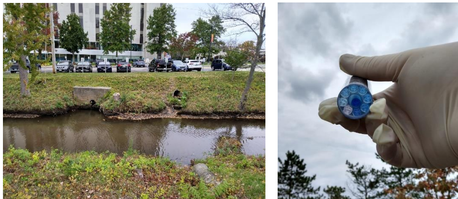
Figure 4: Crosspoint Tower pipes (2.22 on left upstream, 2.21 on right downstream). The right-hand image shows sample 2.21 in the test kit comparator. The sample is in the middle surrounded by a circle of reference tubes.
